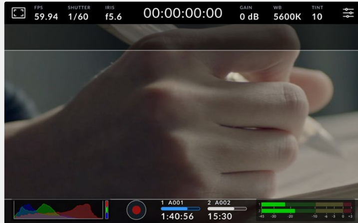
The LCD touchscreen with 2.40:1 frame guides enabled
