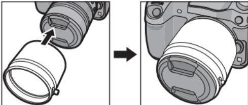
**3 Turn the lens hood screw in the direction of the arrow to fasten the lens hood securely.**
