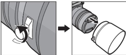
**2 Turn the lens hood around so that it faces the opposite direction, and insert it until it stops.**
