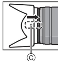
**2** Rotate the lens hood in the direction of the arrow until it clicks and then align the stop mark **(D)** on the longer petal of the lens hood with the mark on the tip of the lens.
