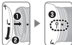
Align the lens hood lock mark (—○) with the lens hood mounting mark (●) on the lens (3).
