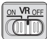
**ON:** The effects of camera shake are reduced while the shutter-release button is pressed halfway and also at the instant the shutter is released. Because vibration is reduced in the viewfinder, auto/manual focusing and exact framing of the subject are easier.
